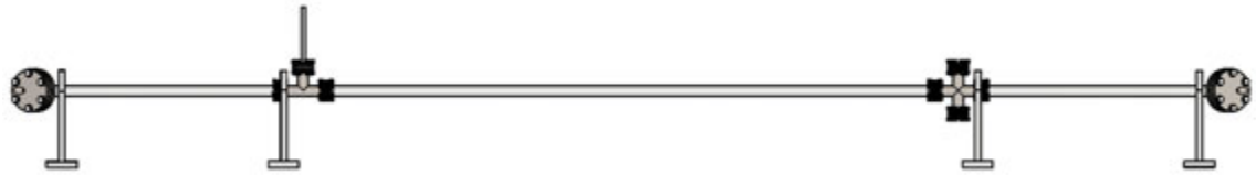
Figure 16: Design 2: The laser enters the fiber from the right and hits the fiber entrance in the center of the cross-shaped part. The tube pointing upwards connects to the vacuum pump and the gas supply.
