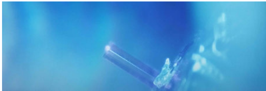
Figure 8: Interface of the thicker fiber, cut under tension with a ruby blade. The picture was taken during the alignment of the laser with the long working distance microscope.
