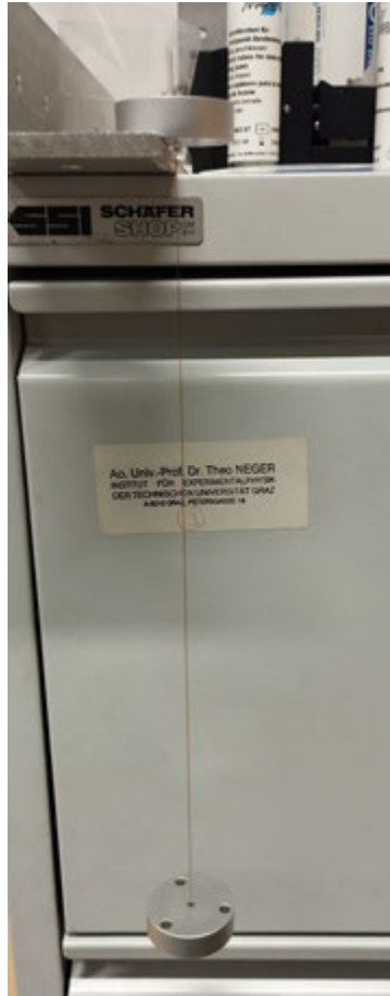
Figure 9: Mounting the fiber to the flanges while hanging vertically.
