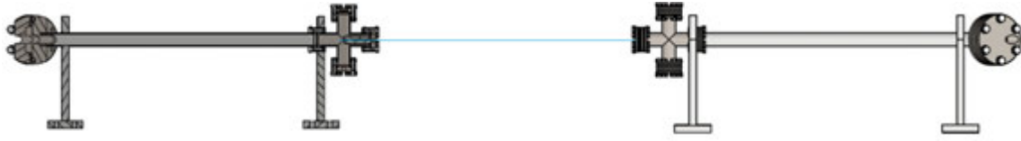
Figure 15: Design 1: Two separate pressure vessels are linked by the fiber represented by the blue line. The left side vessel shows a sectional view. The fiber entrance at the right was positioned underneath a upwards pointing viewport. Via a window in this flange, it was possible to monitor if the laser was aimed directly on the fiber via a CMOS Camera.
