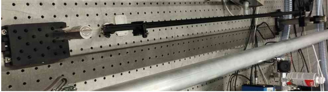
Figure 10: Mounting the fiber under tension to the aluminum profile: On the left side the fiber was glued to an aluminum stand mounted on the stage. On the right side it was fixed onto a static stand.
